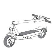
② Put down the front tube, the front tube is automatically locked;
