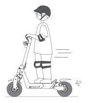
5. To turn, shift your body and turn the handlebar slightly.
