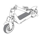
② Put down the folding stem and it will be locked automatically;
