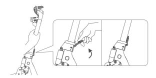
$\ensuremath{\textcircled{1}}$  Hold the folding stem, gently flip down the folding pedal, and bend outwards;
