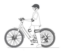
15.Place your other foot on the pedal to keep your feet steady. Focus and keepbalance on yourself, step on the pedal for acceleration. For your safety, the motor won't start until the bike reaches 3.1 MPH (5 km/h).
