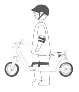
4 The vehicle can be lifted by holding the riser.
